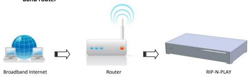
Connect your RIP-N-PLAY to a spare port on your router, using the supplied Ethernet cable.
